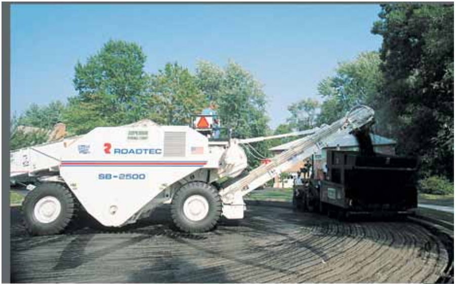
THE SHUTTLE BUGGY® ALLOWS INCREASED PAVER MANEUVERABILITY
