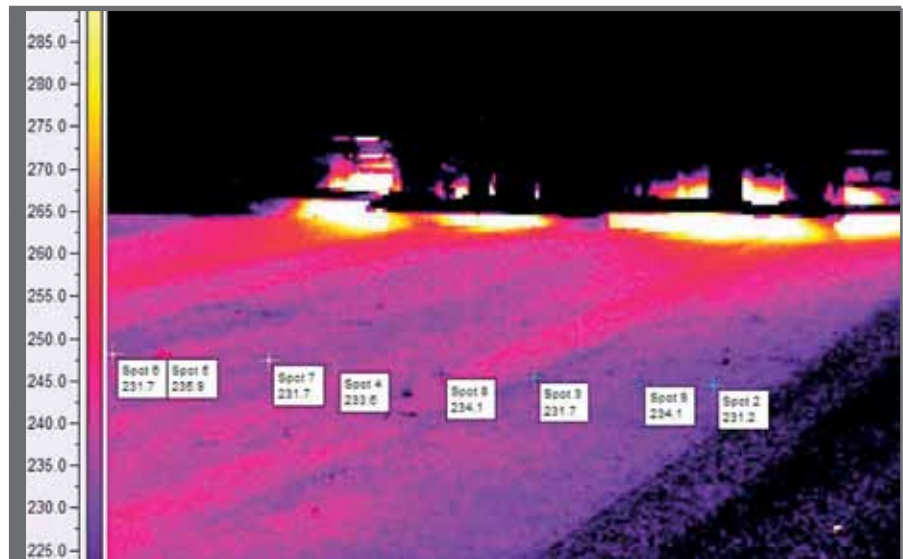
INFRARED IMAGE - PAVER WITH SHUTTLE BUGGY® (WINDROW)
