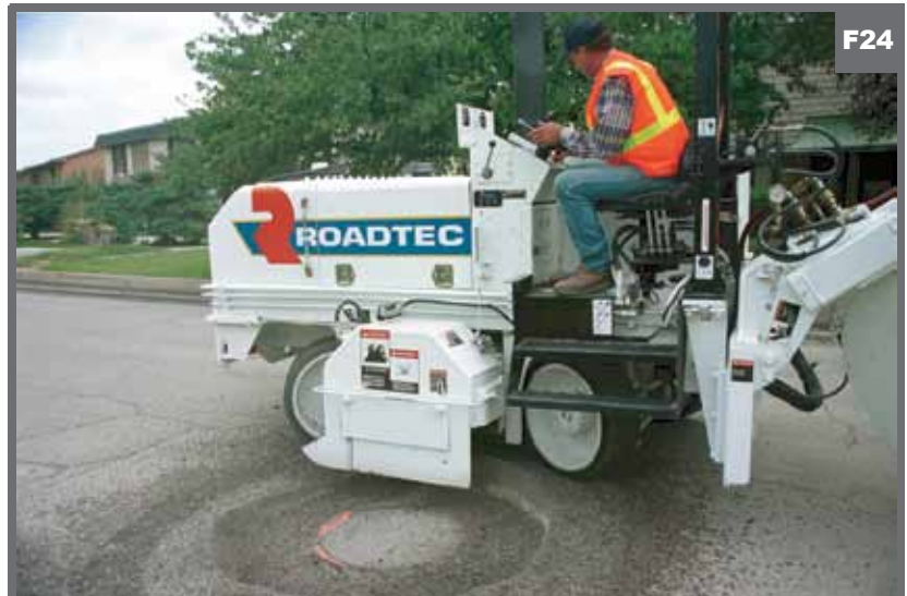
Milling Leaves Utilities Unchanged
