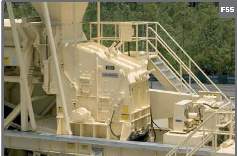
Horizontal Shaft Impactor for High RAP Capacities
