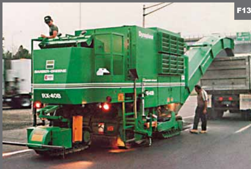
1970's Half-Lane Milling Machine
