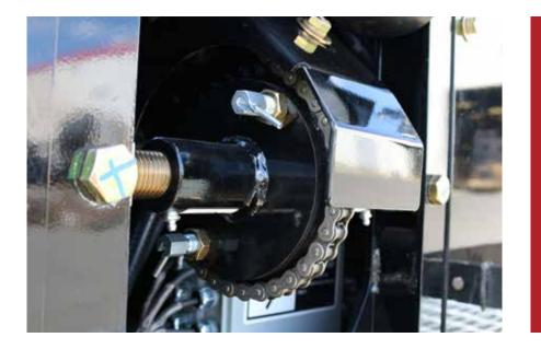
The EZV features a heavy duty, machined power crown assembly with pull pins for adjustment of the lead crown.
